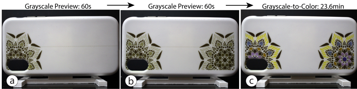
Figure 13: Design iterations on a phone case (iPhone XR). (a) The designer drafts one mandala on the phone case and transfers it using the grayscale preview function. They iterate on the design and add a second mandala in 60 seconds (b). The designers is satisfied with this version and transfers the preview texture to a full color texture (c).
