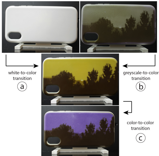
Figure 6: Color-to-color transition: saturating individual pixels with the UV projector enables us to update from (a) white-to-color, (b) monochromatic-to-color, and (c) color-to-color textures.
