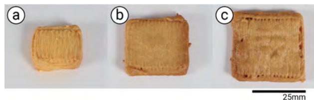
Figure 4. Varying infill density, which also varies size: (a) 70% infill (25x25mm), (b) 55% infill (35x35x5mm) and (c) 39% infill (40x40mm). All cookies are printed with 5mm height.
