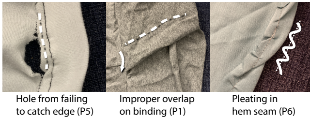
Figure 5: Several participants made errors after choosing to ignore practice steps suggested by InStitches. P5 skipped the practice for the armhole binding and failed to catch the edge of the shirt with the binding strip, creating a hole. P1 did not practice the armhole binding either and ended up with improper overlap in the underarm area. Instead of sewing a smooth bottom hem, P6 created several unintentional pleats after not practicing this step.
