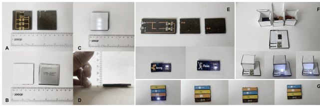
Figure 4: Electronic magnetic sheet: (A) Exposed PCBs of sheets A and B (B) Display and battery sides. (C) When the complementary sheets A and B combine, the LEDs light up and blink every second. (D) The thickness of the electronic magnetic sheet is 3mm. (E) Application: Authentication User Interface. Two PCBs, here labeled Tom and Jerry, will selectively pair in different configurations on the larger bottom PCB, lighting up different LEDs with Tom and Jerry IDs. (F) Application: Object classification. Three magnetically-folded boxes of equal size contain different contents. A classifier that couples the magnetic interactions to a force transducer communicates the contents of the boxes via LEDs without opening them. (G) Tangible Interface for learning the Scratch language. Scratch components will only bond in locations where they form correct semantic meanings, and light up an LED when placed there to communicate this to the student.
