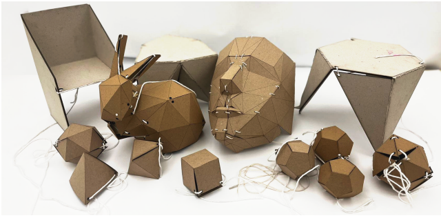
Figure 6: Structures fabricated using our pipeline range from regular polyhedra to organic shapes, and from load-bearing to aesthetic, across a range of scales, for applications that include VR, education and functional load-bearing contexts.
